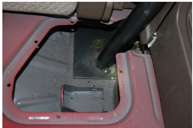
Figure 3 Driver C Pillar Mounting Plate
