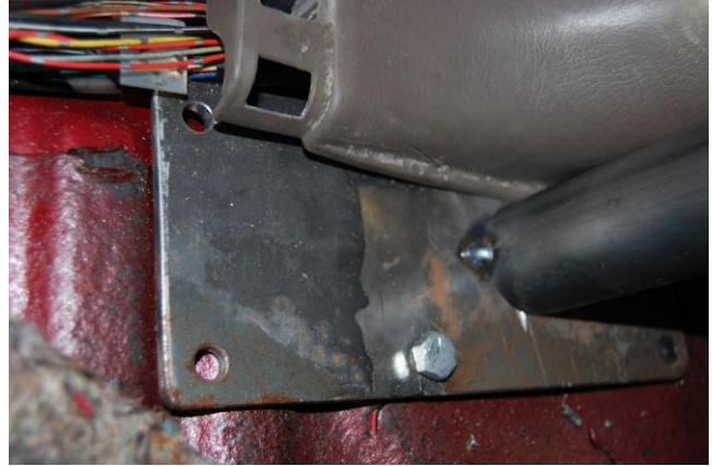
Figure 1 Driver Side A Pillar Mounting Plate
