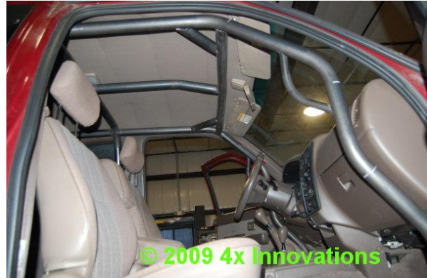
Figure 6 Front of cage detail
