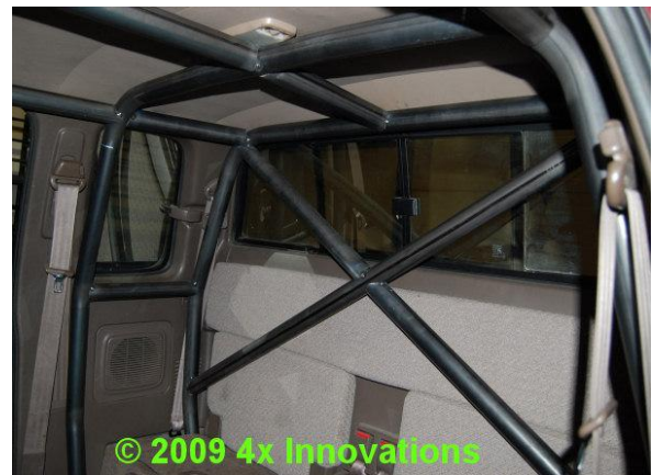
Figure 5 B and C pillar detail
