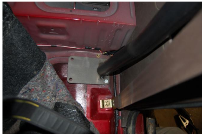
Figure 2 Driver Side B Pillar Mounting Plate
