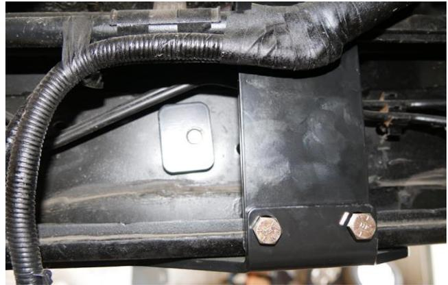
Figure 11 – Driver electrical box Square nut position
