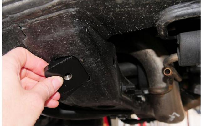
Figure 8 – Inserting square nut into the cross member
