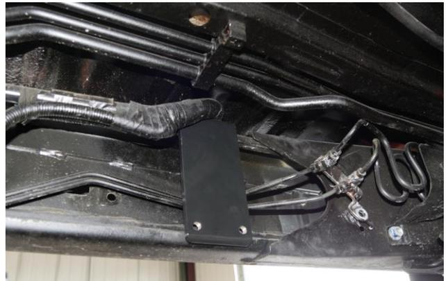
Figure 9 – Driver Front Inner Frame Brace in place
