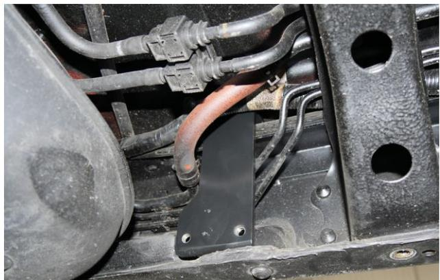
Figure 10 – Driver Rear Inner Frame Brace in place
