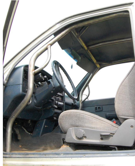
Fig 8 – A pillar, front cross and front center location
