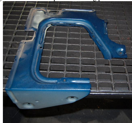
Fig 6 – C pillar plate seat ledge piece to be removed
