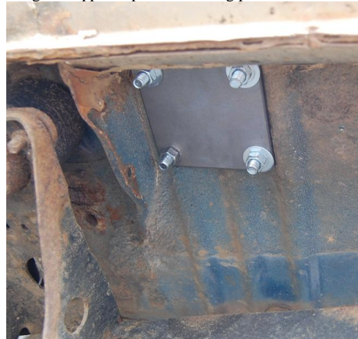
Fig 2 – Lower A pillar mounting plate orientation
