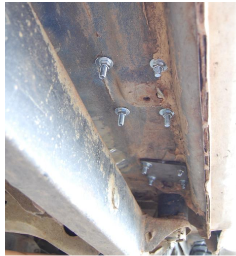
Fig 5 – Lower B & C pillar mounting plate orientation
