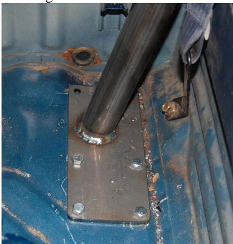
Fig 4 – Upper C pillar mounting plate orientation
