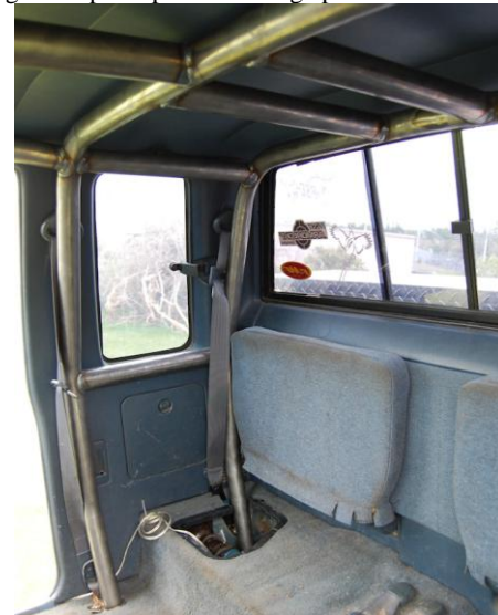
Fig 7 – B to C pillar connection tubes
