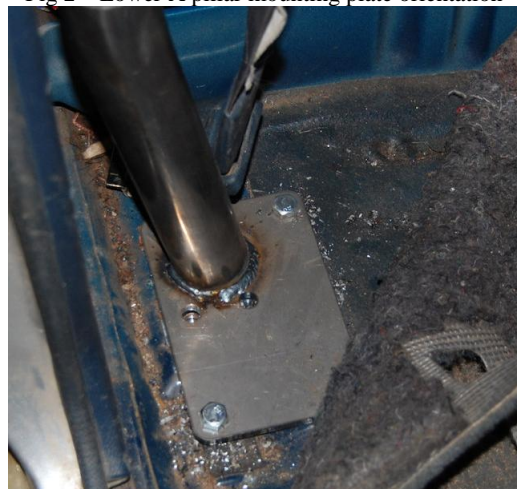
Fig 3 – B pillar mounting plate location
