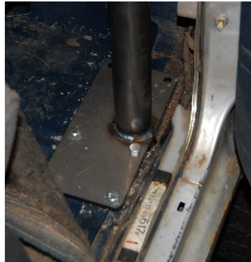
Fig 1 – Upper A pillar mounting plate orientation
