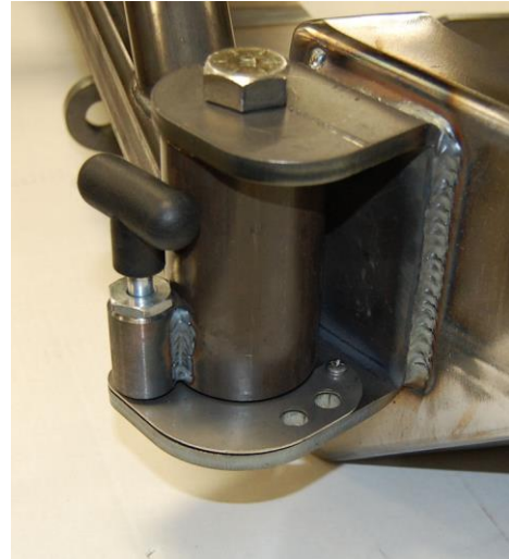
Figure 3. Tire Carrier Pivot Hinge Assembly
