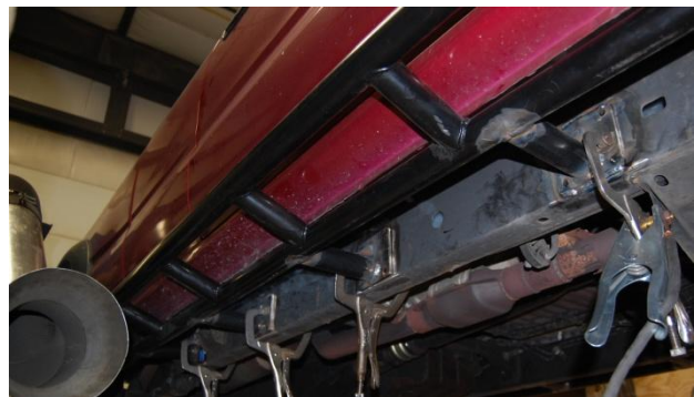
Figure 2. Rock Slider held in place with clamps for welding.
